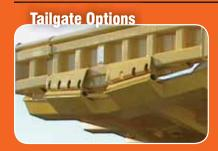
**Rubber Cushion Pads** are recommended for underground operations and operations with high road speeds or uneven haul roads. Shown at left, Cushion Pads reduce wear, bouncing and noise and often increase the life of your PHIL Autogate<sup>®</sup> Tailgate. These may be installed on an existing gate or purchased with the tailgate.
