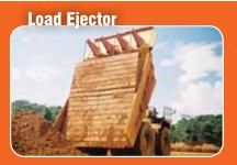
The PHIL Load Ejector dislodges sticky material clinging or sticking to the truck body through a series of overlapping, jointed steel plates attached to the top of the front slope plate and extending down the body floor. In the dump cycle, the Load Ejector slides away from body floor, hanging vertically or nearly vertically, to dislodge sticky material.
